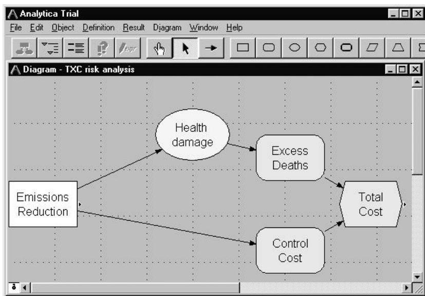
Figure 10.2. An early stage in the creation of the influence diagram, that is shown in final form in Figure 10.1. The analyst, using the Analytica diagram editor, is starting to fill in variables between the decision on the left and the objective on the right.
