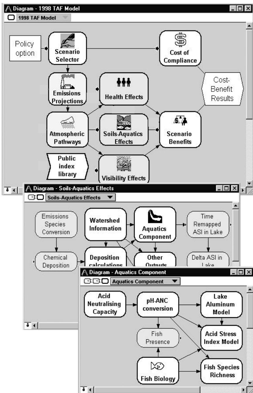
Figure 10.4. Three influence diagrams showing three levels of the module hierarchy for the TAF model. A mouse click in a module opens a diagram to show lower level details.
