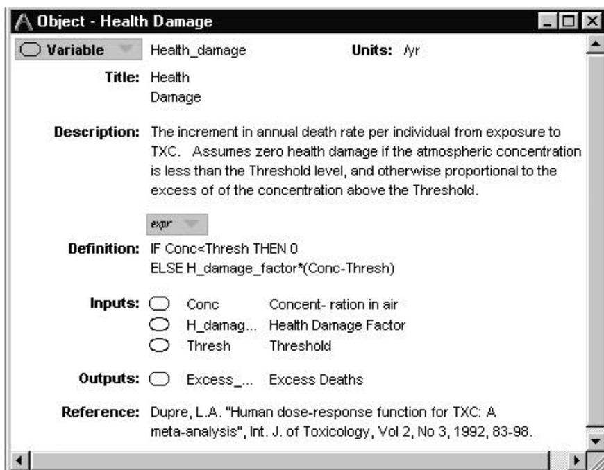
Figure 10.3 An Object card showing detailed information about the variable, Health Damage. The inputs are the variables that appear in the definition above, and also linked in by influence arrows in the influence diagram in Figure 10.1. The reference field may give a bibliographic reference, as in this case, or a name or contact for the source of the relationship, number, or probability distribution.
